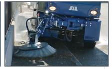
Exclusive capability to sweep in unbalanced conditions (ex. sidewalks). The system allows to sweep on bumps with no operator's action required (optional).
