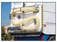
Rear powerful wandering vacuum hose, 6 m lenght -140 mm diameter. High pressure washing system (140÷200bar) w. spray-gun and 12m-hose reel.
