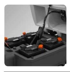
The detergent water tank serves as battery compartment, allowing the housing of great capacity batteries granting continuous working time up. Large capacity shock and acid proof polyethylene tank (1101) improves productivity avoiding frequent refilling and idle time.
