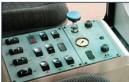
Easy-to-use keypads to operate the machine. "EasyStart" single button for all required functions on/off.
