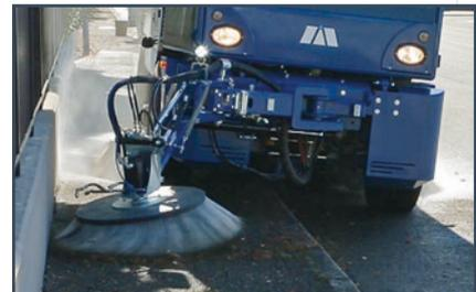
Exclusive capability to sweep in unbalanced conditions (ex. sidewalks). The system allows to sweep on bumps with no operator's action required (optional).
